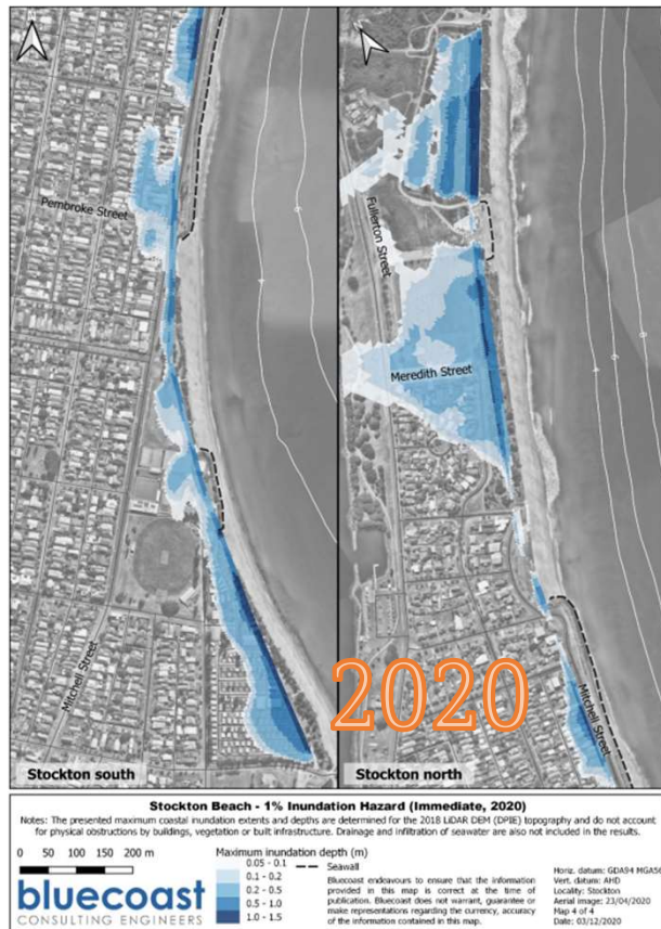
Figure 11: Coastal inundation hazard for 1%AEP in 2020 (immediate).
